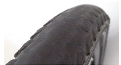
Tread is worn out. Rubber is still present. This tire could still be ridden.
