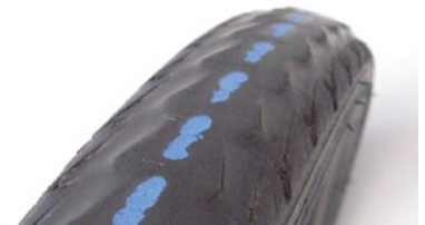
The puncture protection layer can be seen. The tire must be changed urgently.
